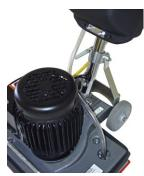
Solution is applied to the pad when released by a manual trigger on the 4 gallon solution tank. (high speed model)
